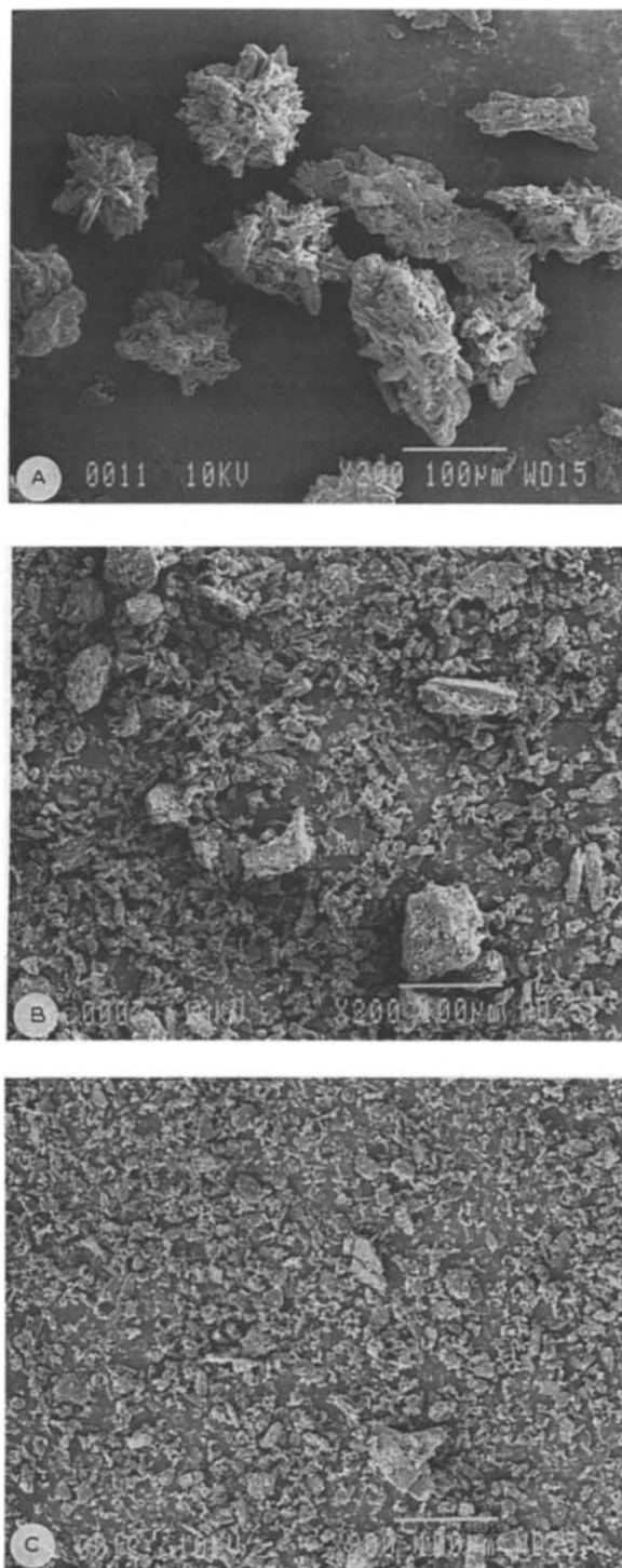
Fig. 2. Scanning electron micrographs of unmilled (A), once-milled (B), and twice-milled (C) drug. SEMs courtesy of J.D. Gagliardo.
